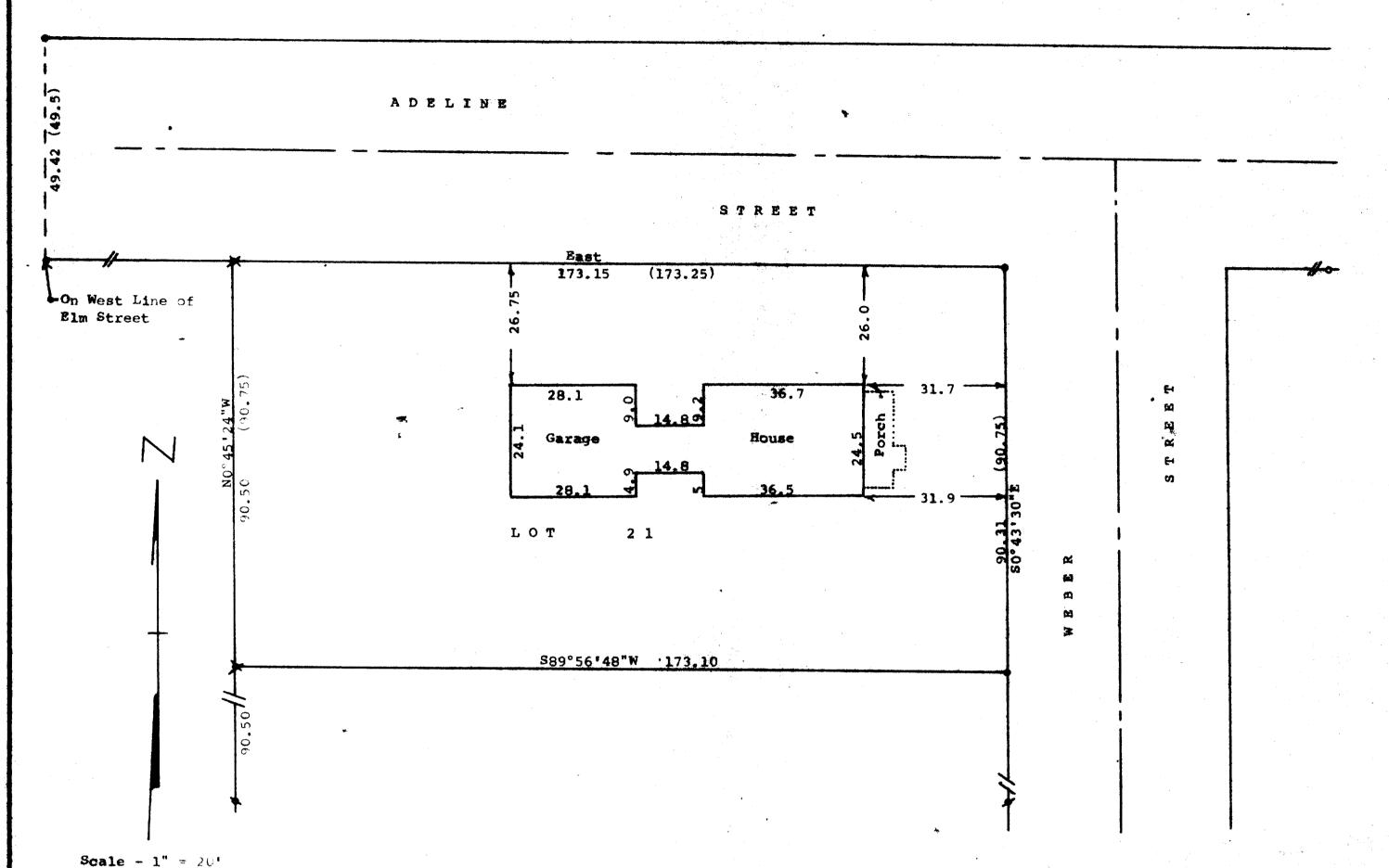
• 3/8" Iron Rod Set # 3/4" Iron Pine Found • 3" X 24" Iron Pipe Set X= 14" X 24" Iron Pipe Set " 1" Iron Pipe Found Survey ordered by: Churchill Real Estate Walworth, WI 53184 Bearings referenced to the assumed bearing of East along the southline of Adeline Street
